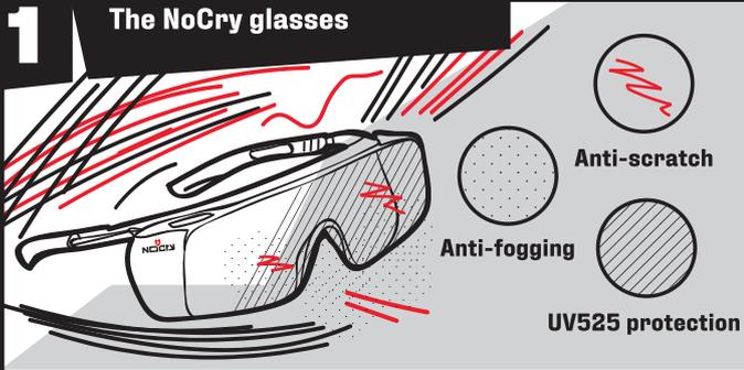
The lenses have UV525 protection against blue light up to 525nm along with anti-fog and anti-scratch treatments.
